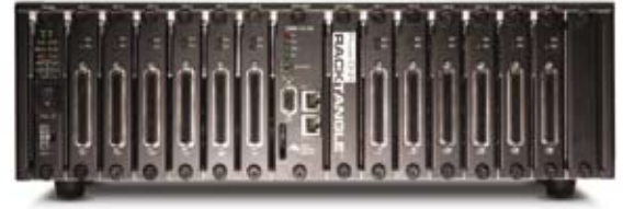
DNR-12-1G includes rack/chassis, Dual channel NIC, CPU, Dual USB 2.0 ports, Buffer Board, Power Supply, and software. Optional slot covers for empty slots. are also available.
