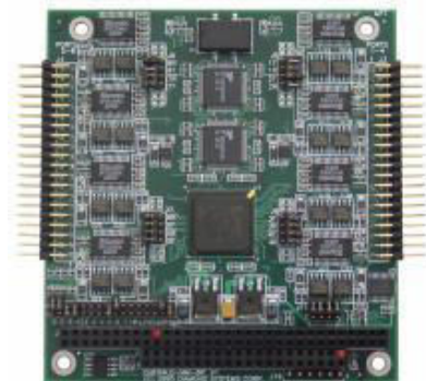
Diamond Systems Europe GmbH Programmable Serial Ports unit in use at JPADS controls
