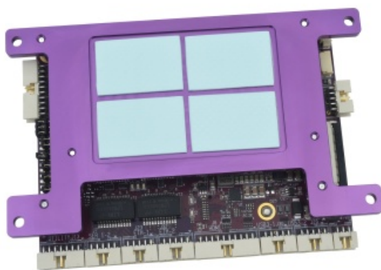
Heat spreader mounting plate provides improved heat dissipation
