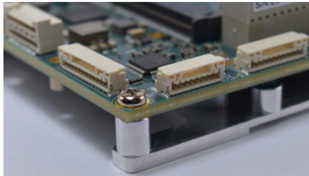
Thicker PCB inhibits flexing from high vibration
