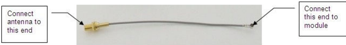
Figure 29: GPS Transition Cable
