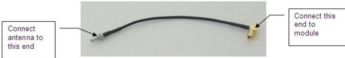
Figure 27: Old GPS Transition Cable
